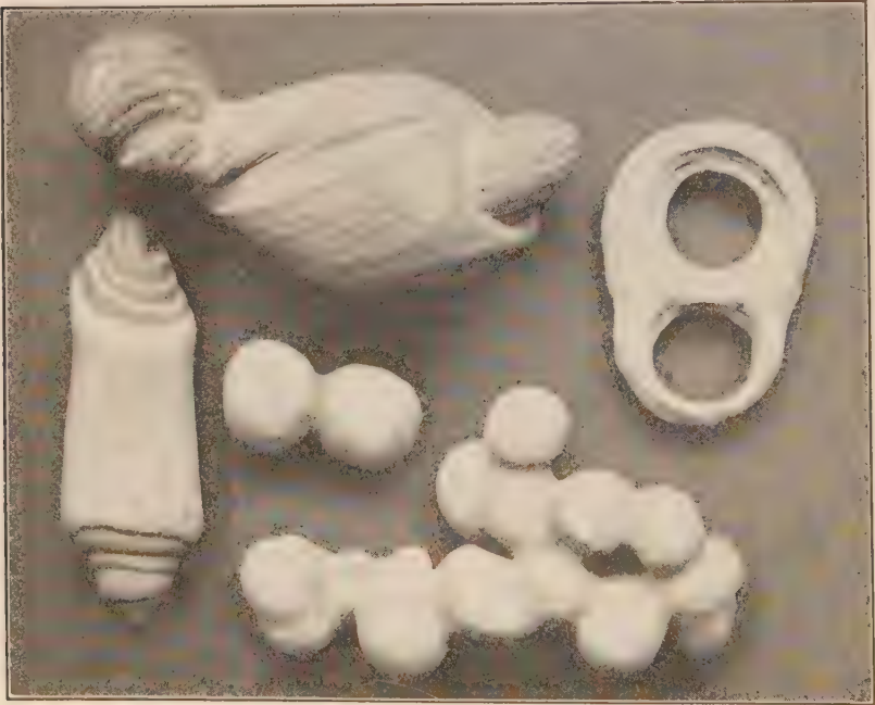
FIG. 55. — Clay-stone concretions of various shapes. They are composed largely of lime carbonate and occur in clay.
